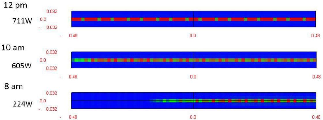
Figure 4 False color representation of the radiation falling onto the receiver (red indicates the highest intensity) for 8 am, 10 am and 12 m during the equinox.
