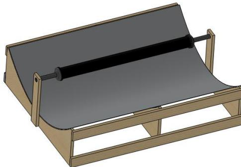
Figure 3. 3D render of the conceptual design of the semi-static solar concentrator.
