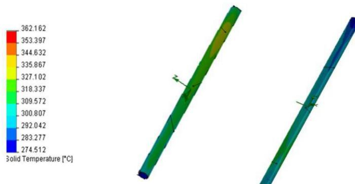
Figure 7 Temperature distribution as calculated for a copper receiver with evacuated tube cover assuming a heating power of  $900 \text{ W}$  uniformly distributed.
