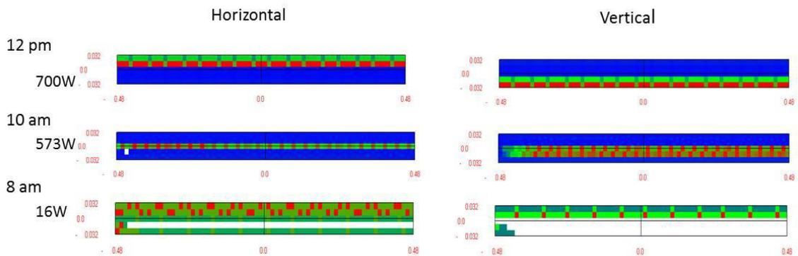
Figure 5 False color representation of the radiation falling onto the receiver ( red indicates the highest intensity) for 8 am, 10 am and 12 m during the solstice.
