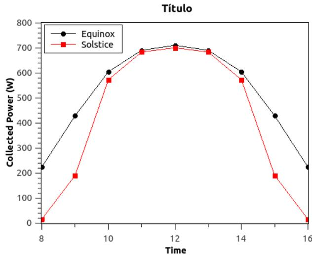
Figure 6 Instant collected power for the designed receiver, assuming a clear day with  $900 \text{ W/m}^2$  irradiance at noon, (black) for the equinox, (red) for the solstice.
